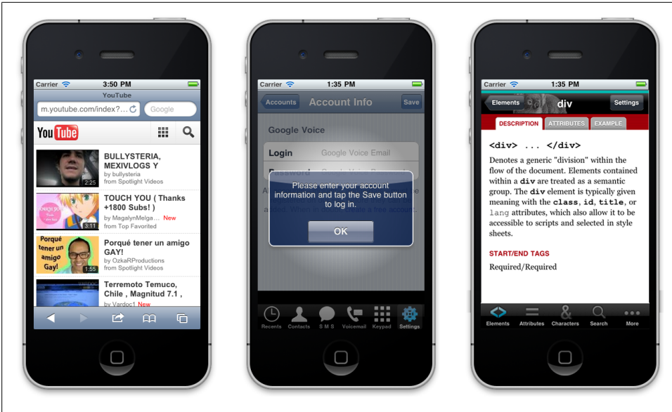
Figure 1-1. A webapp delivered as (from left to right) a browser-based experience, a full-screen installed application, and an embedded webapp inside a native app (hybrid)
