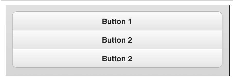
Figure 3-18. When we have different inline buttons, it's better to wrap them in a control group for better appearance
