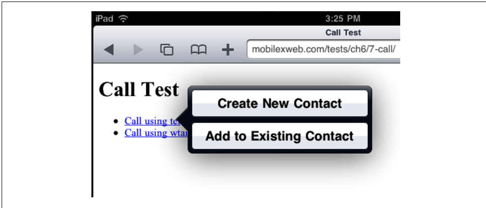
Figure 2-18. Some devices, such as Apple's iPad, don't have calling capabilities but they offer other choices with a tel link
